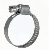
5/16"(8mm) Mini worm drive hose clamp can be easily installed in restricted space because it is small and light. It is also called American type hose clamp. 8mm band can generate significant sealing pressure with relatively low installation torque. Save cost and space.
